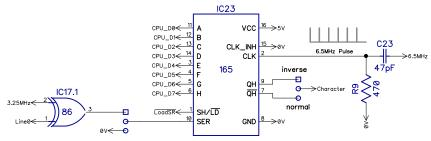
Characters can be inverted by setting bit 7 of the character code. This is latched at the same time as the data is latched into the shift register. During optimisation, this has been implemented using some left over gates, hence the slightly unusual design. A counter is used, if the invert signal is set, there will be a single pulse which will set the output high. Each memory request cycle, the counter will be reset.
