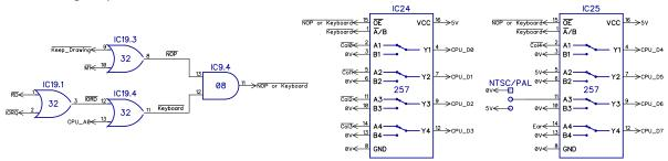
The keyboard is read using bits 0-4 of the input port. There are five column lines, which are pulled high normally. When the keyboard is being scanned, the upper eight address lines are set so that one is low at a time. If a key is pressed on the 5x8 crosspoint keyboard on that row, the column line reads low.
