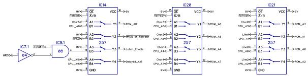
The lower three bits are generated from a line counter, this counts up each line, and is reset on a vertical sync so it is always on line 0 at the start.
